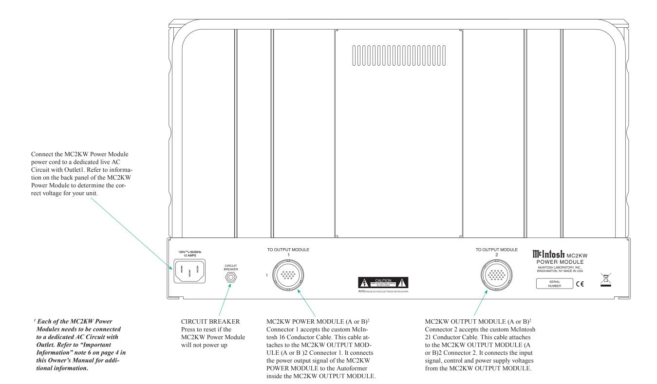
Modules "A" and "B" connect to the same MC2KW Output Module.
